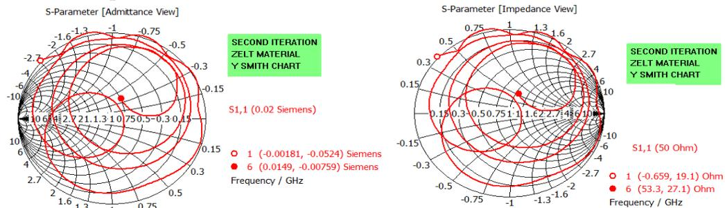
Figure 11 Admittance Result and Impedance Result of second Iteration for Zelt Material
