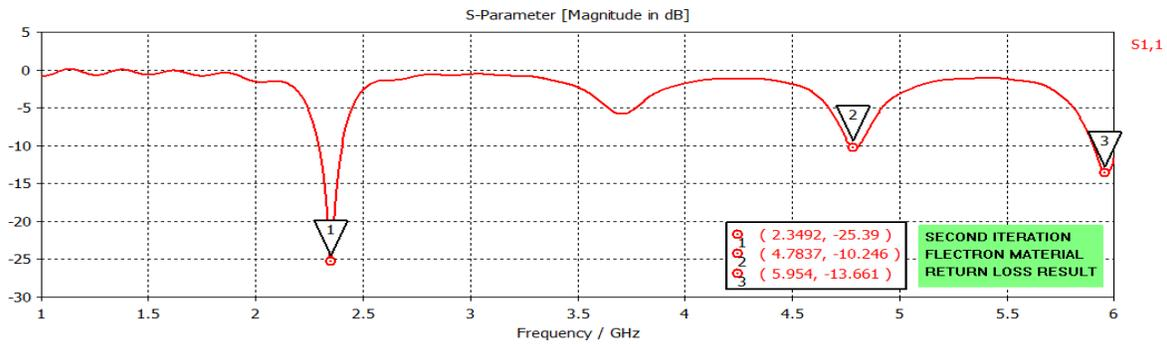
Figure 19 Return loss Result of second Iteration for Electron Material
