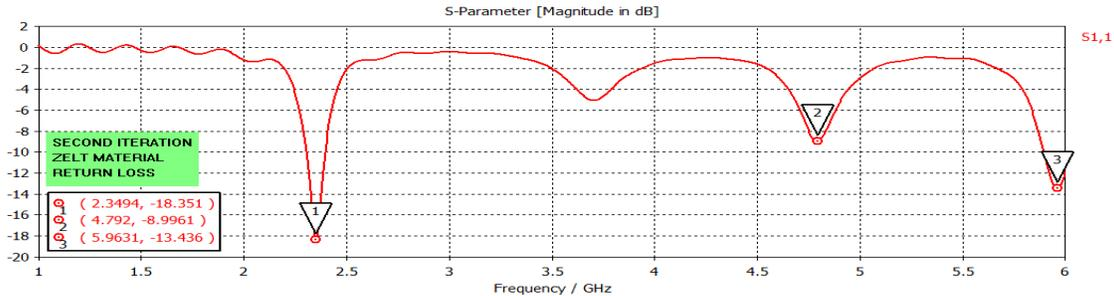
Figure 12 Return loss Result of second Iteration for Zelt Material
