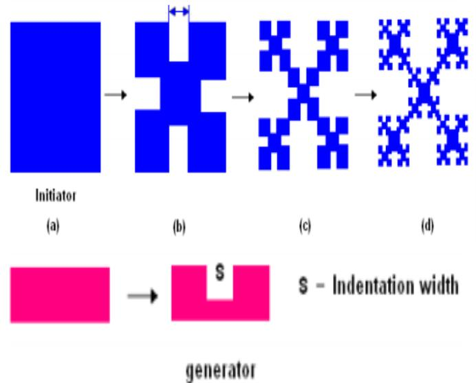
**Figure 4 Generation of Minkowski fractal patch antenna (a) Initiator patch (b) First iterated Minkowski fractal patch (c) Second iterated Minkowski fractal patch (d) Third iterated Minkowski fractal patch.**
