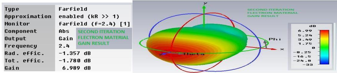
Figure 14 Gain Result of second Iteration for Electron Material
