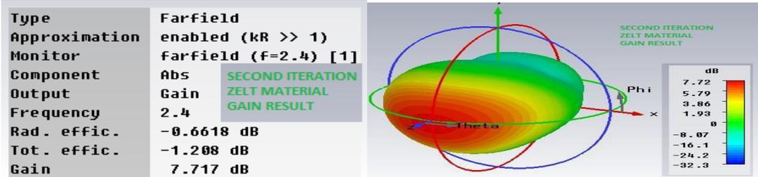
Figure 6 Gain Result of second Iteration for Zelt Material
