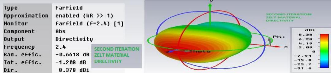
Figure 7 Directivity Result of second Iteration for Zelt Material
