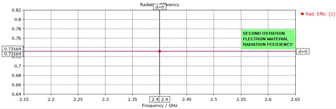
Figure 18 Radiation efficiency Result of second Iteration for Electron Material
