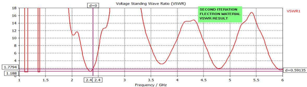
Figure 16 VSWR Result of second Iteration for Electron Material
