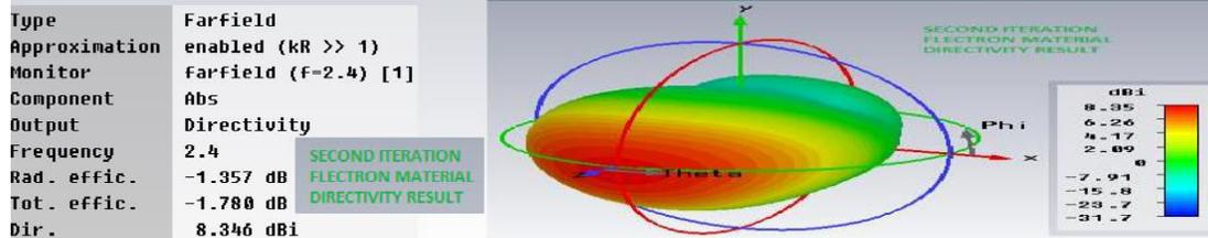
Figure 15 Directivity Result of second Iteration for Electron Material
