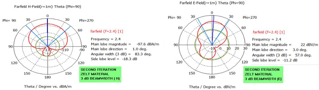
Figure 5 3 dB Beam Width H-Field and E-Field Result of second Iteration for Zelt Material
