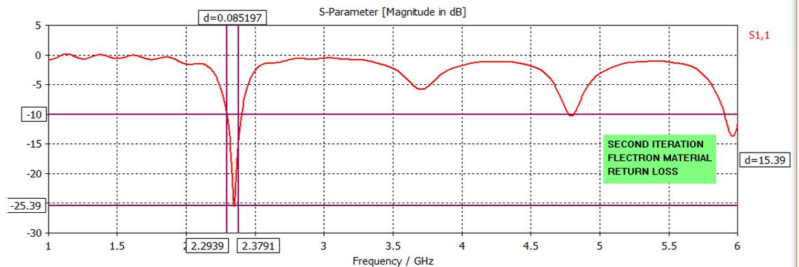
Figure 20 Return loss Result of second Iteration for Electron Material
